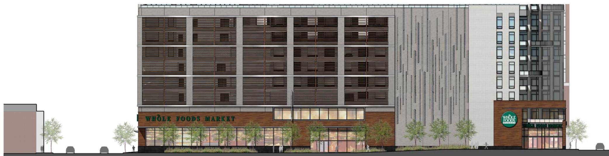
S. CENTRAL AVE - WEST ELEVATION- OPTION C WHITE BRICK EXPANDED NO METAL PANEL REVEAL B/W WHITE & GREY MASONRY
