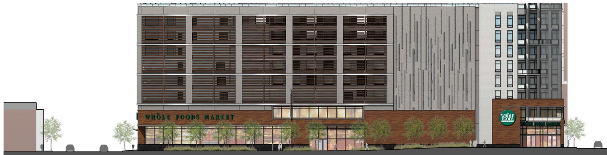
S. CENTRAL AVE - WEST ELEVATION- OPTION B WOOD BASE EXTENDED AT GROUND
