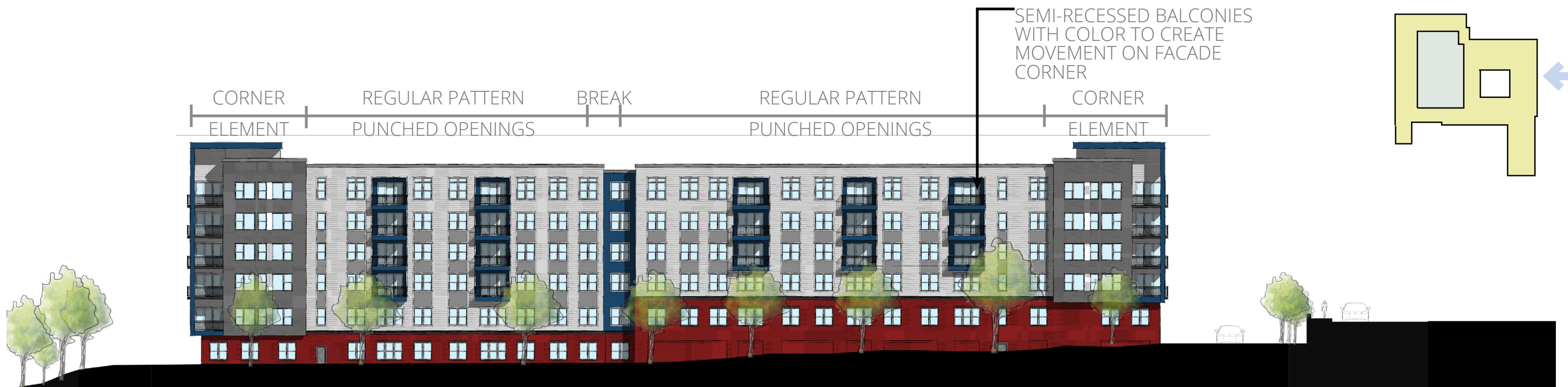
EAST ELEVATION BUILDING ELEVATIONS
