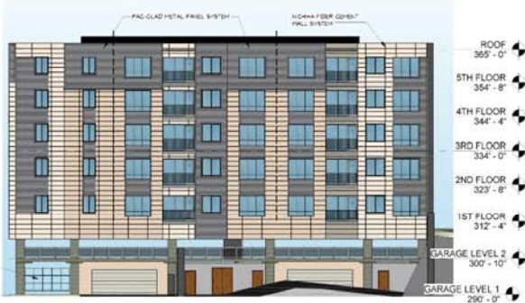
3 EAST ELEVATION - PRELIM
