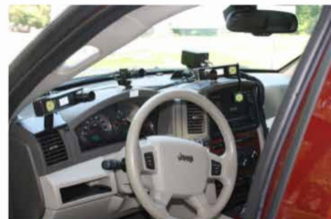
Figure 1. Eye tracking system camera placement.
