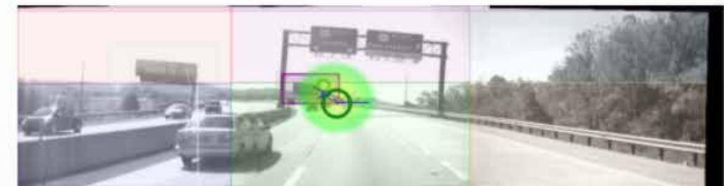
Figure 21. Heat map near the middle of a DCZ for a standard billboard in the daytime on a freeway.
