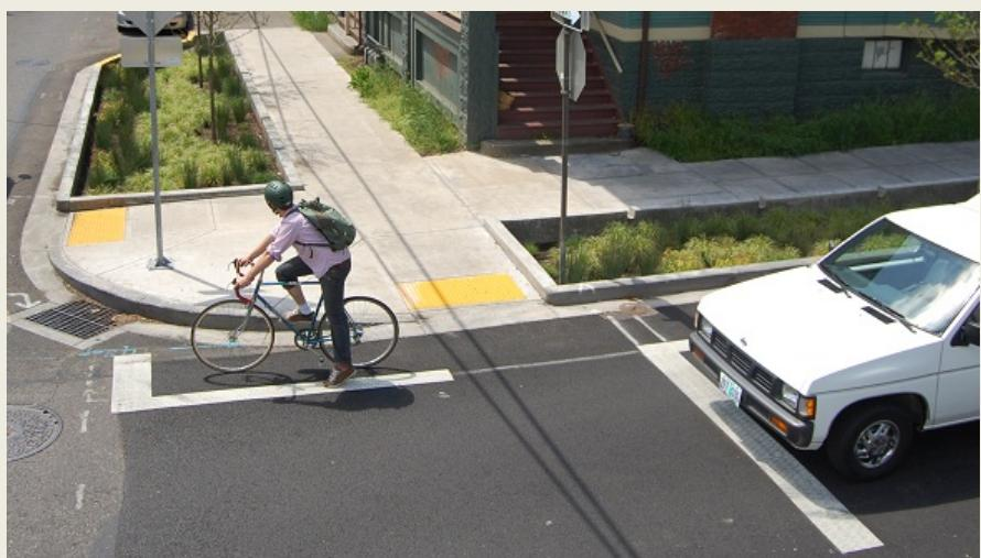
*Photo 25: Sample curb extension with bioretention facilities and expanded pedestrian ramps*
