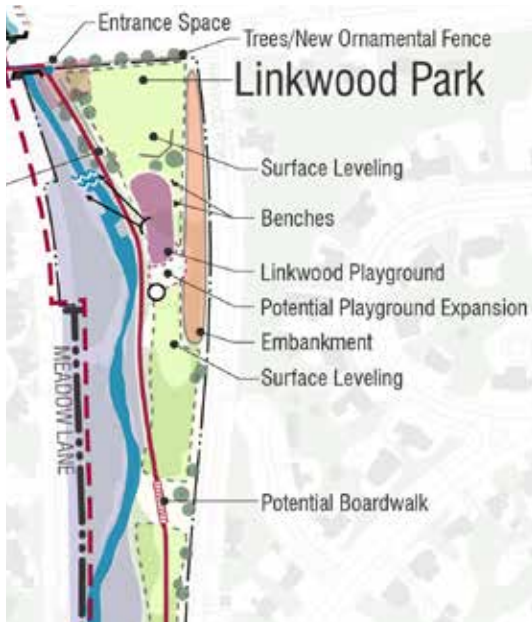
Detailed plan of Linkwood Park recommendations. Refer to Overall Plan for a legend.
