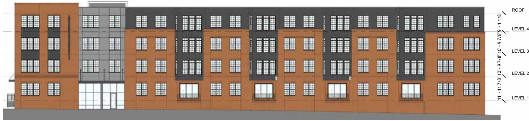
1 WEST ELEVATION ALONG S BOND ST
